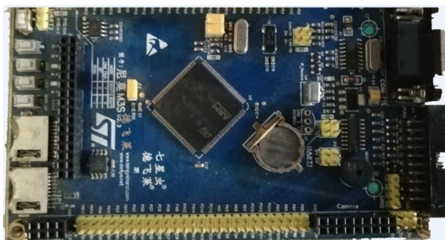
Fig. 2. STM32F103ZET6 development board
