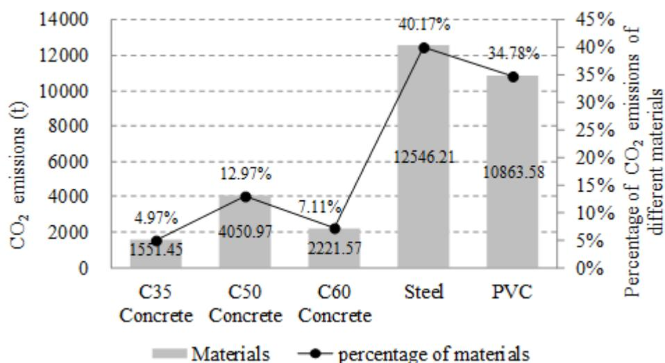
Fig. 2 CO<sub>2</sub> emissions of different materials in Zhuguang Road Tunnel during the raw material production stage
