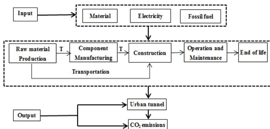
Fig. 1 The scope of CO<sub>2</sub> emissions of the life cycle of prefabricated urban tunnel
