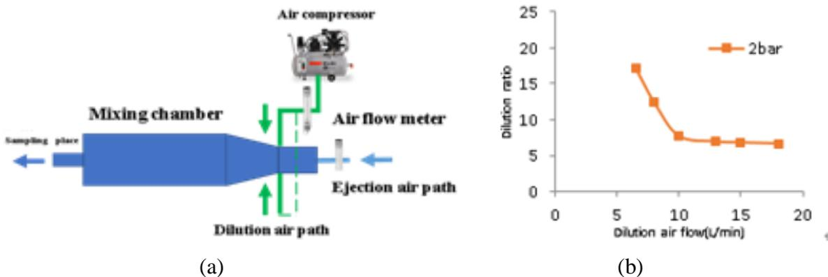
Fig. 2 Schematic diagram of the experiment system and the experimental results
