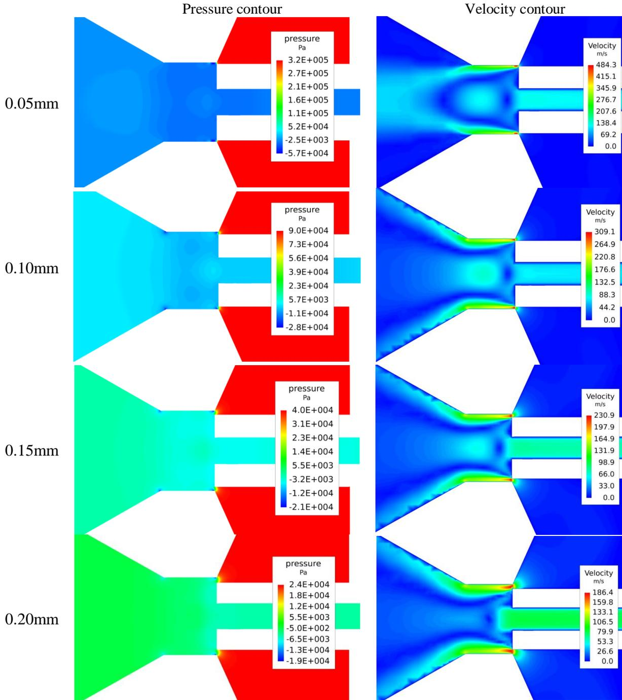
Fig. 6 Pressure and velocity contours under different gap width
