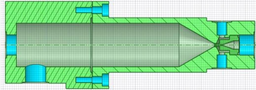
Fig. 1 Geometric model of the diluter
