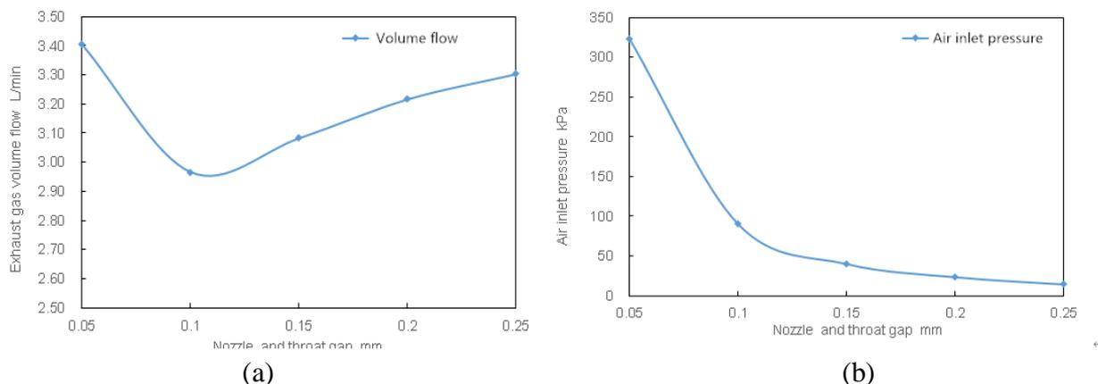
Fig. 7 The relationship between exhaust gas flow / compressed air inlet pressure and clearance
