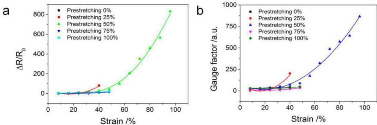
Figure 3. Tensile test of GNP/AS-3 strain sensor in the range of 0-100% pre-tension (a) Resistance change rate comparison chart and (b) Sensitivity comparison chart
