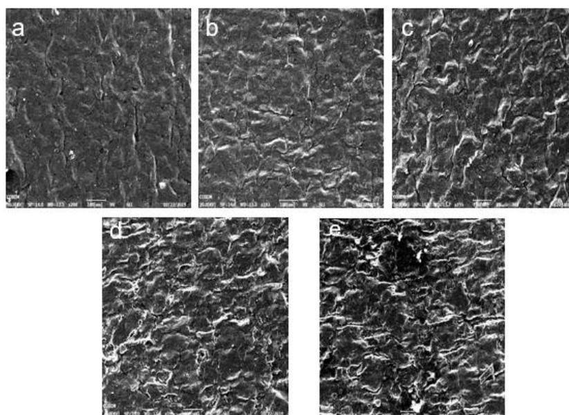
Figure 2. GNP/AS-3 strain sensor tensile (a) 0%, (b) 20%, (c) 40%, (d) 60%, (e) 80% strain SEM images
