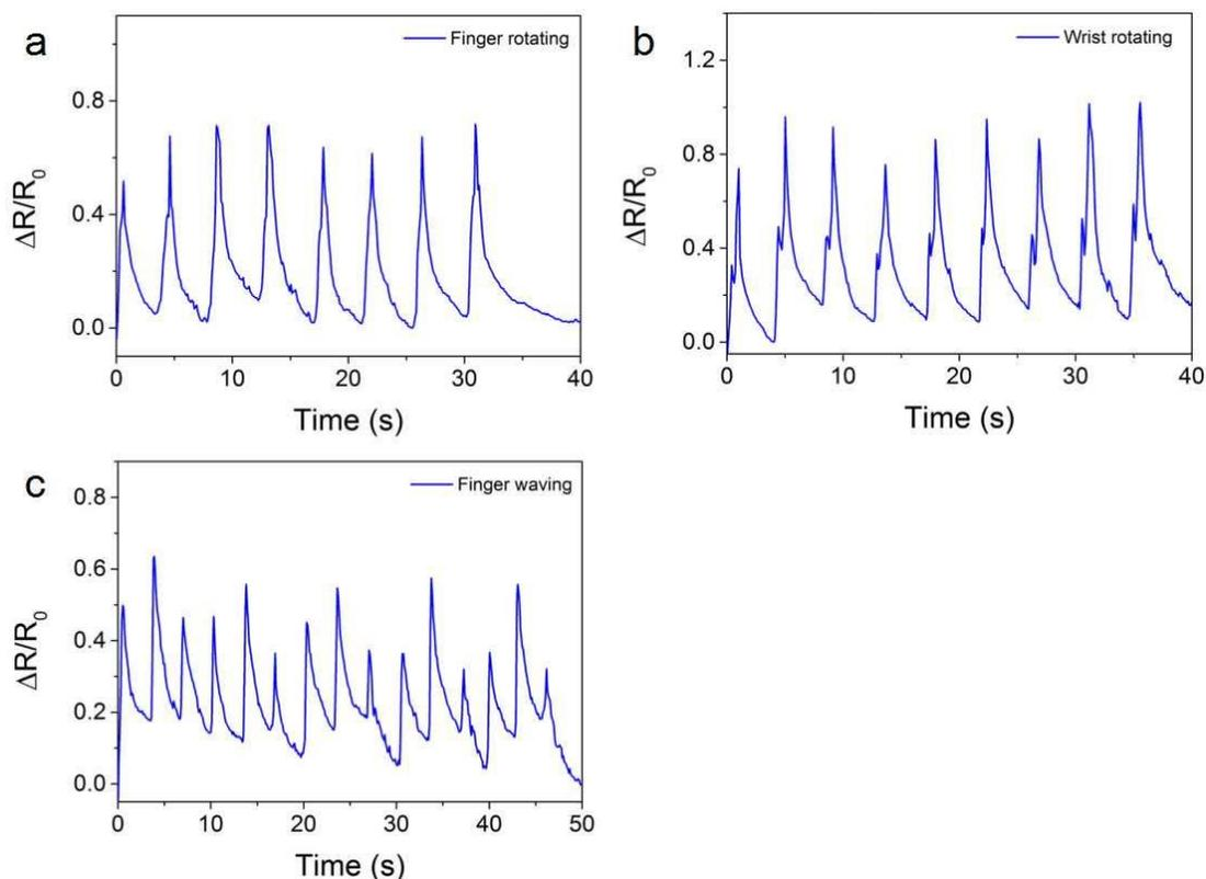
Figure 5. GNP/AS strain sensor (a) finger joint rotation, (b) wrist joint rotation, (c) finger swing repetitive action resistance change rate response graph
