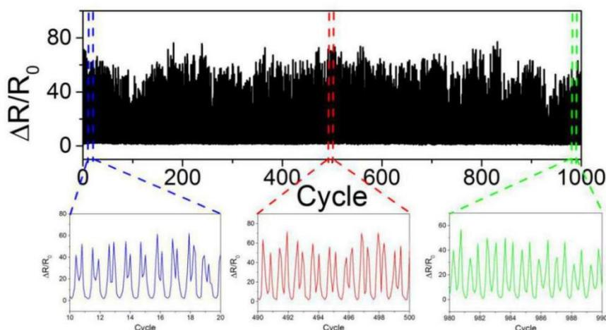
Figure 4. Test of 0-10% strain resistance change rate of pre-stretched 50% GNP/AS-3 strain sensor
