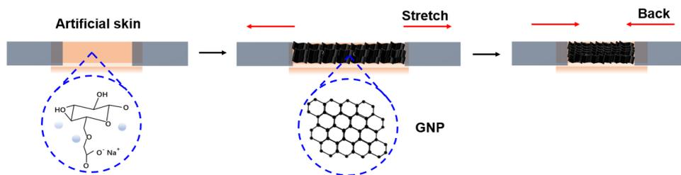
Figure 1. Schematic diagram of the preparation process of GNP/AS flexible strain sensor
