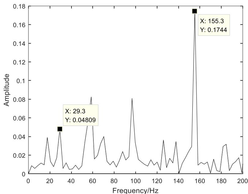
Fig. 4 Envelope spectrum of inner ring fault reconstruction signal
