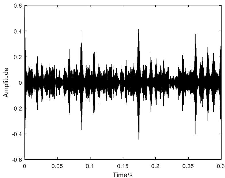
Fig. 5 Outer ring fault reconstruction signal
