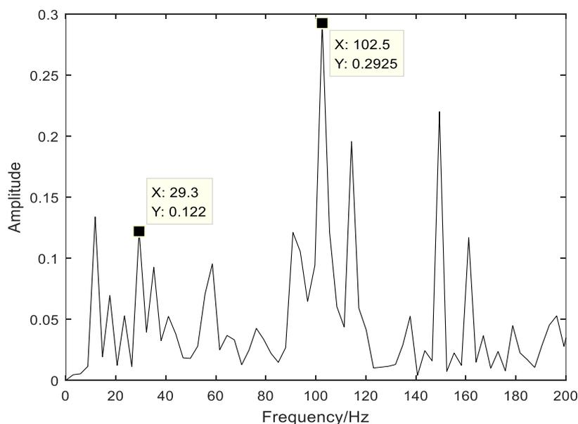
Fig. 6 Envelope spectrum of outer ring fault reconstruction signal
