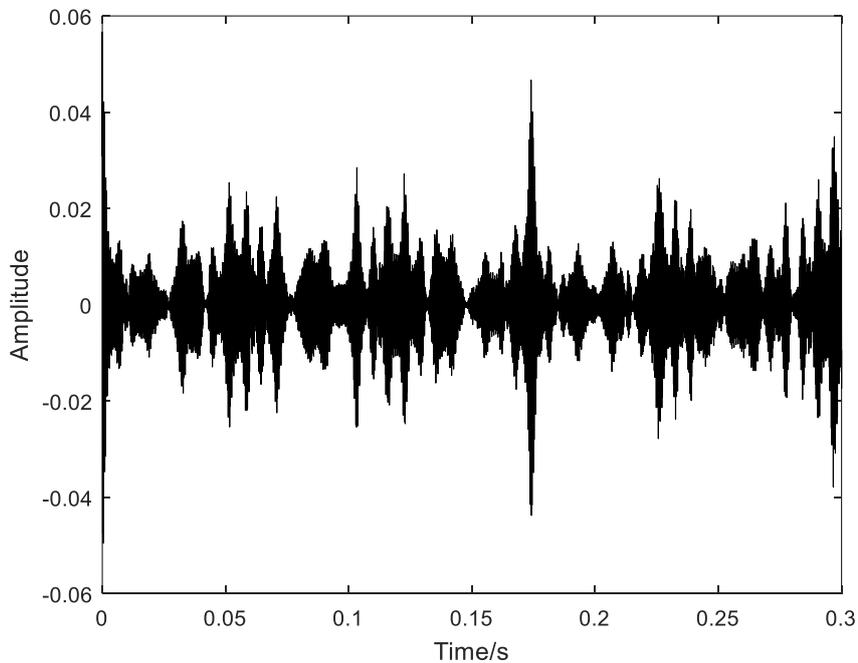
Fig. 3 Inner ring fault reconstruction signal
