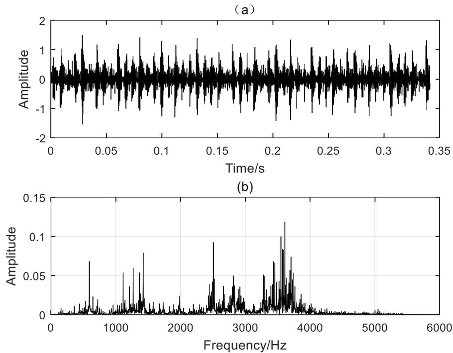
Fig. 1 (a) and (b) are time domain and frequency domain characteristics of inner ring signal respectively
