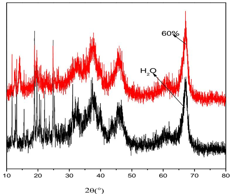
Fig. 1 XRD patterns of alumina
