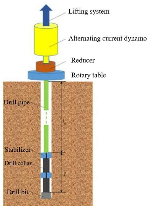
**Fig. 1** Dynamic model of the drill-string system
