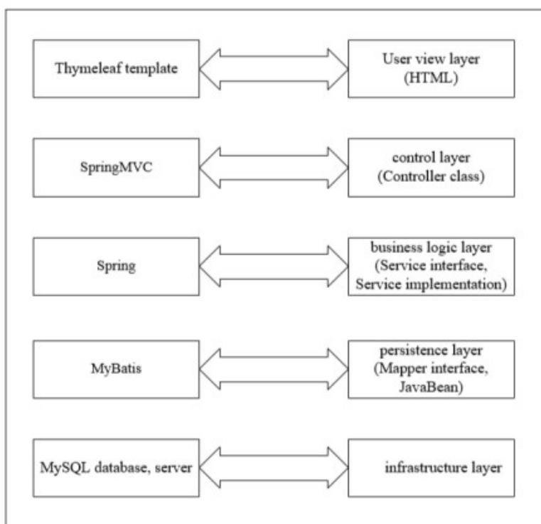
Fig. 2 System Design Architecture Diagram
