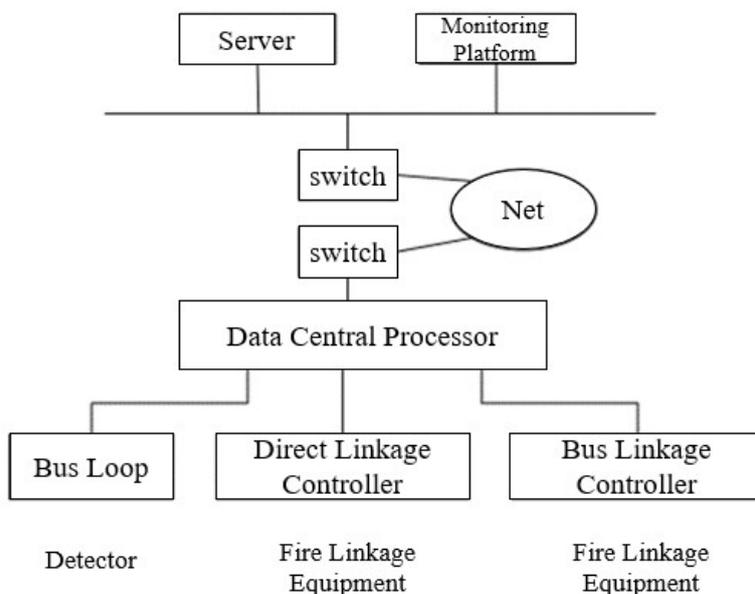
**Figure 1.** Multi-feature intelligent perception system structure
