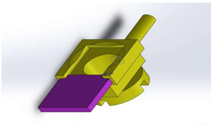
**Fig. 5** Oil collecting head and sealing sheet
