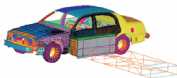
Fig 1. Finite element model of vehicle side impact
