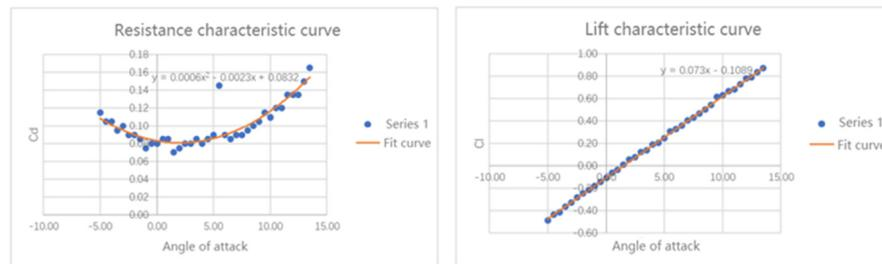
**Fig 3.** Resistance characteristic curve and lift characteristic curve of unmanned aerial vehicle
