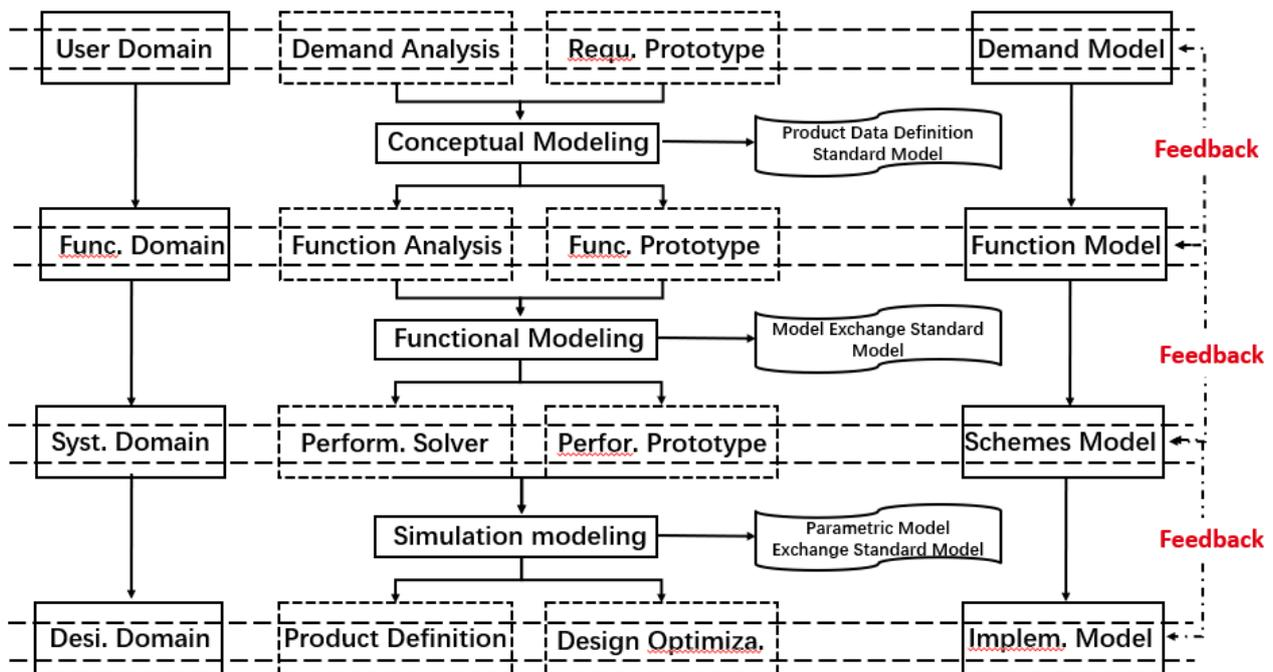
**Fig 1.** The division process of complex product design stages
