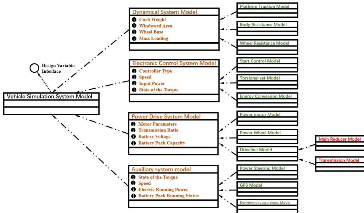
**Fig 5. Vehicle Hierarchical Module Structure Model**
