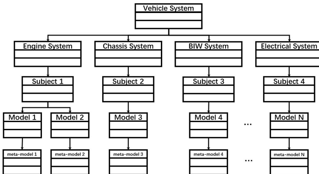
Fig 2. A Metamodel-Based Multidisciplinary System Decomposition Model
