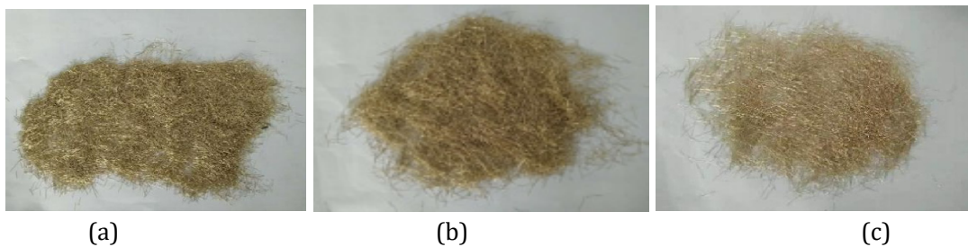
a-6mmCopper coated steel fiber; b-13mmCopper coated steel fiber; c-17mmCopper coated steel fiber
