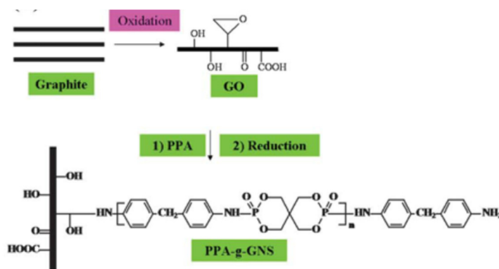
Fig 4. Preparation process of PPA-g-GNS
