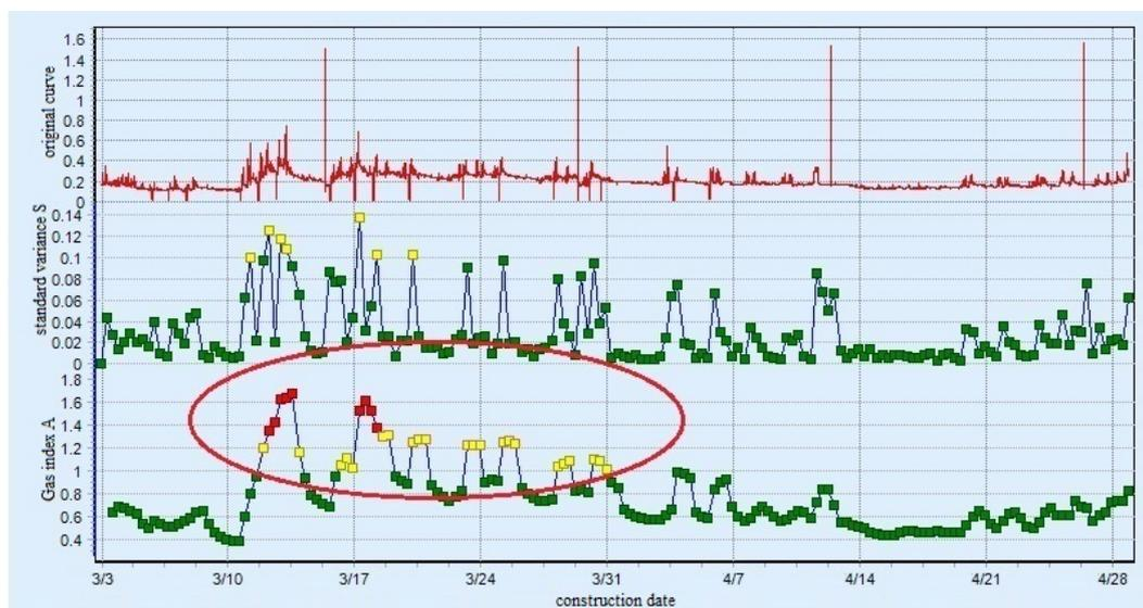
**Figure 6.** Example diagram of gas gushing warning
