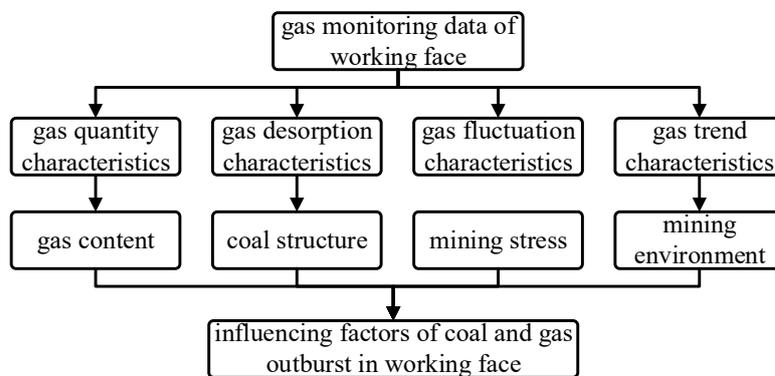
Figure 4. The structure of gas gushing and outstanding danger
