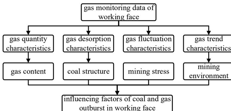
Figure 4. The structure of gas gushing and outstanding danger
